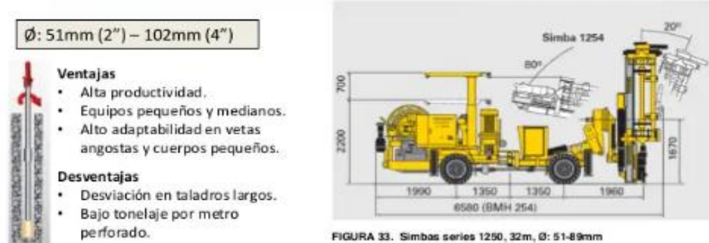
FIGURA 33. Simbas series 1250, 32m, Ø: 51-89mm
