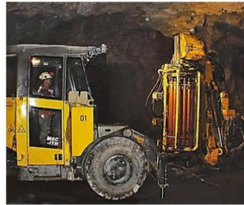
FIGURA 36. Simba M6C – DTH, 51m, \varnothing : 95-165mm
