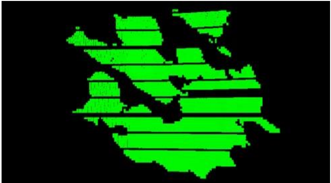
Figura 7. Solido Resultante del MSO (Mineable Shape Optimizer) – Veta Gisela
