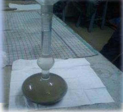
A Lechatelier flask, a specialized glass flask used for testing concrete, sitting on a white cloth on a tiled floor. |
