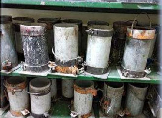
A collection of various concrete molds of different shapes and sizes, arranged on a green metal shelf.      |
