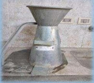
A metal Abrams cone, a funnel-shaped mold used for casting concrete, standing on a tiled floor.                        |
